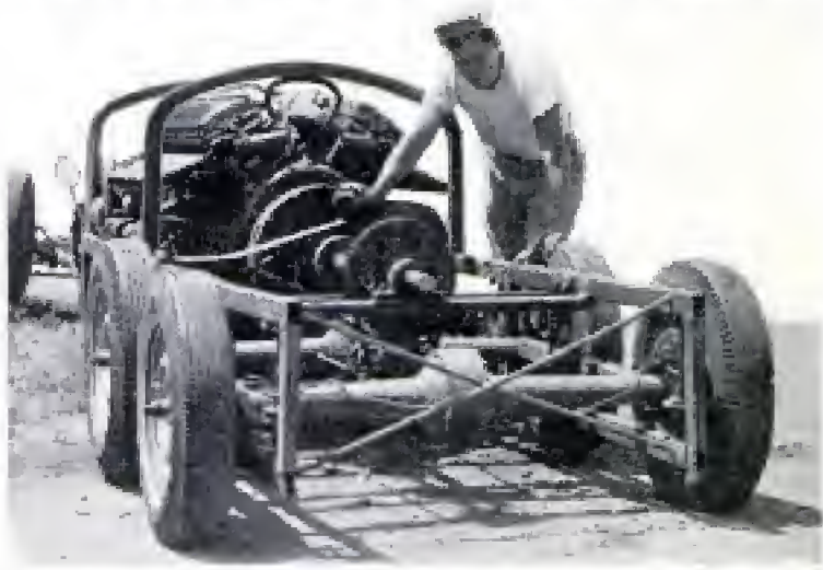
Tandem-wheel drive increases the traction and minimizes the tendency to "fishtail." Car has a clutch from a 30-ton tank
